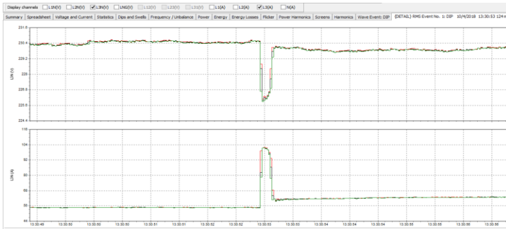
Fig 11 Voltage dip event while using cranes
